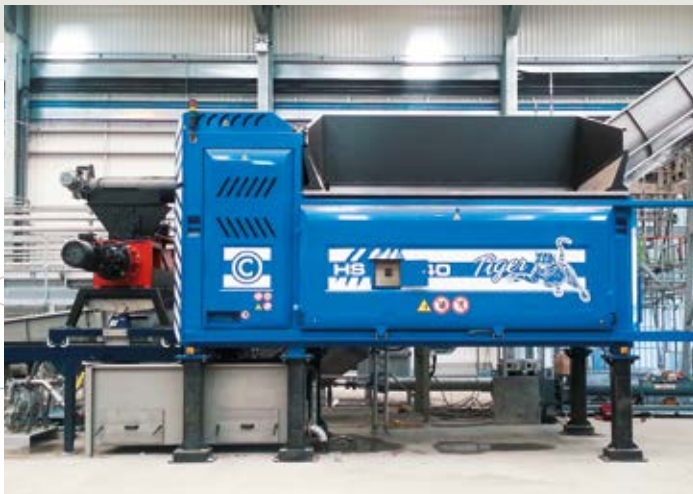
TIGER DEPACK HS 640 (ENGLAND) / ORGANIC FRACTION OF URBAN SOLID WASTE FROM DIFFERENTIATED WASTE DISPOSAL
